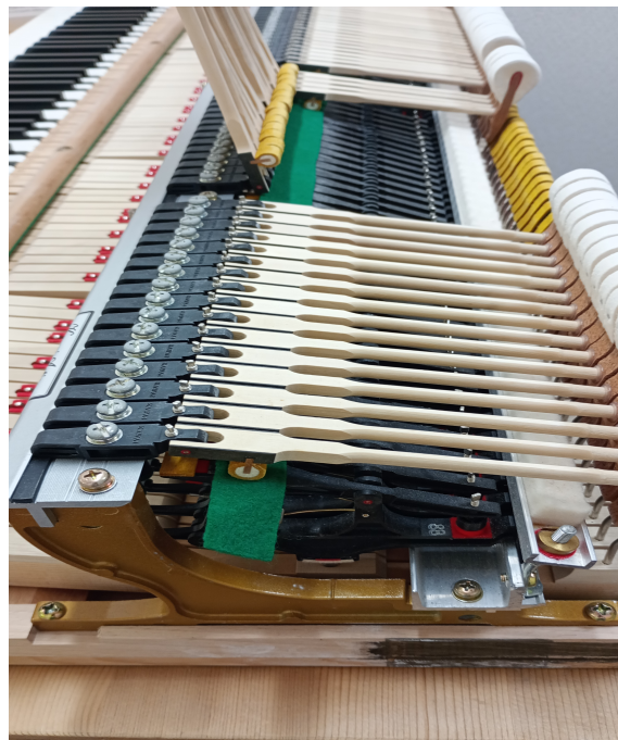
Figure 5: Felt strips under rollers raise hammers towards strings.
